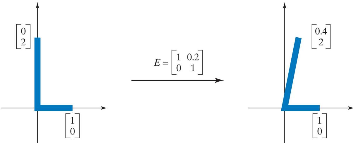
The foot of the L remains unchanged, while the back is shifted horizontally to the right; the L is italicized, becoming *L*. We will call this transformation a *horizontal shear*.
