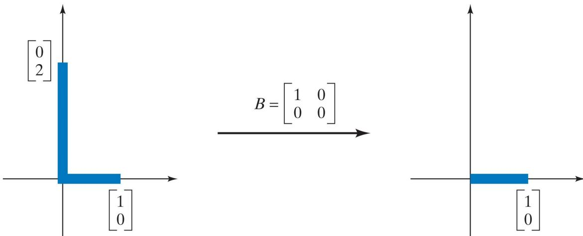
The L gets smashed into the horizontal axis. We will call this transformation the *orthogonal projection onto the horizontal axis*.
