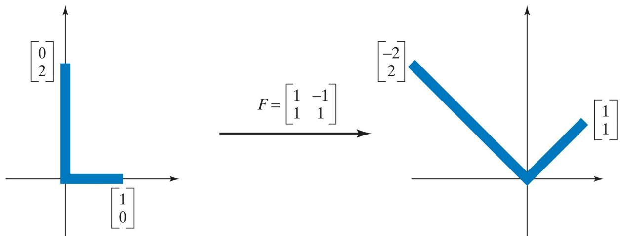
There are two things going on here: The L is rotated through  $45^\circ$  and also enlarged (scaled) by a factor of  $\sqrt{2}$ . This is a *rotation combined with a scaling* (you may perform the two transformations in either order).
